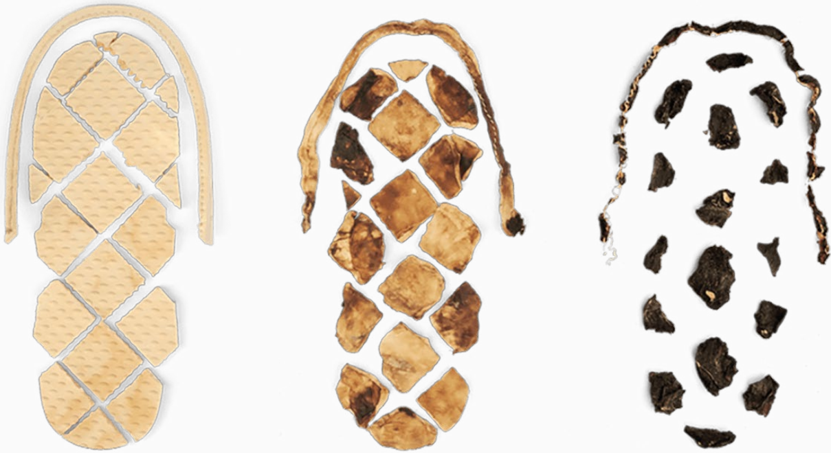
A visual demonstrating Forager's stages of decomposition when discarded in optimal conditions. Source: Ecovative
